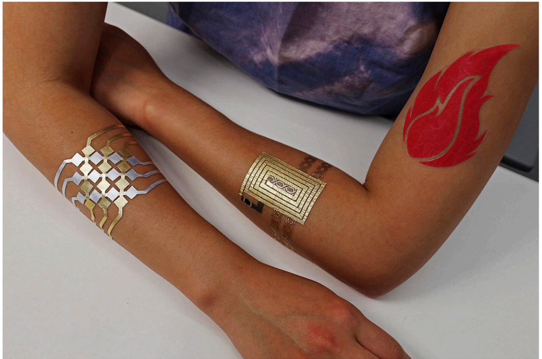
Inspired by the trend of metallic tattoo art, the researchers behind DuoSkin designed a process for making gold-leaf temporary tattoos that can function like a track pad, communicate information wirelessly, or change color with body temperature. Image courtesy of Jimmy Day/MIT Media Lab.
